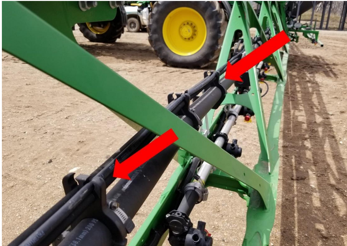
Fig. 7: Power Cable Routing Along Boom
