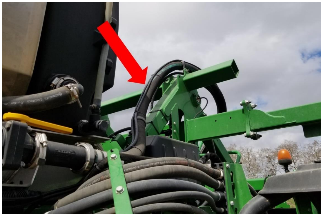
Fig. 9: Power Cable Routing Along Main Supply Hose
