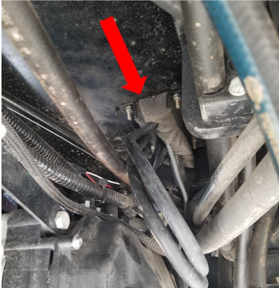
Fig. 10: Cable Entry On Underside of Cab Floor (Case IH Patriot)
