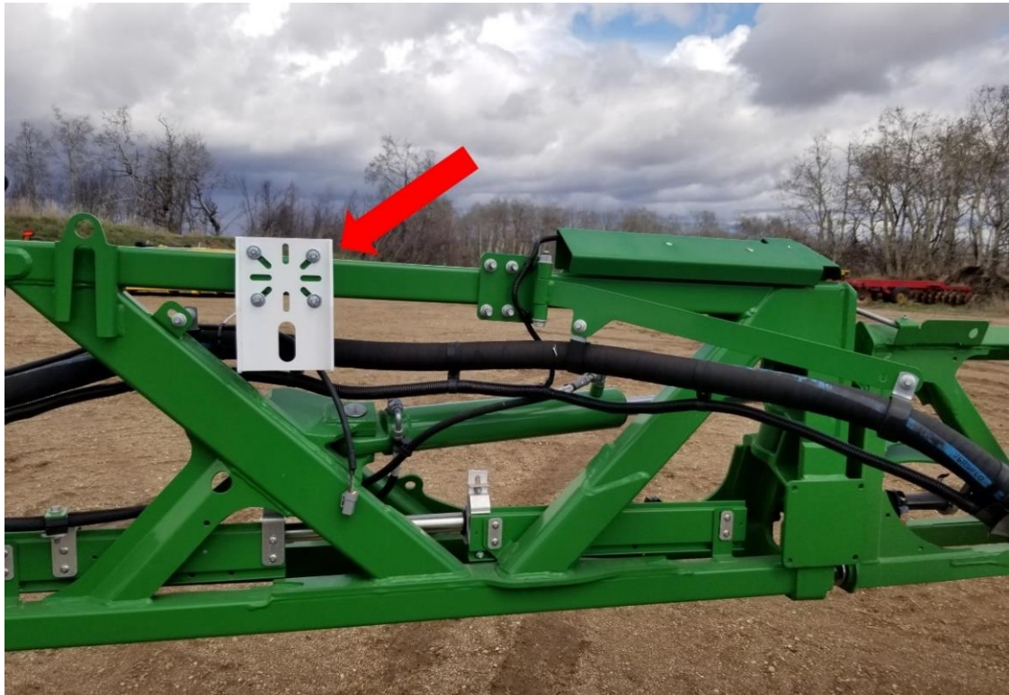
Fig. 3: Mount Location at Top of Boom
