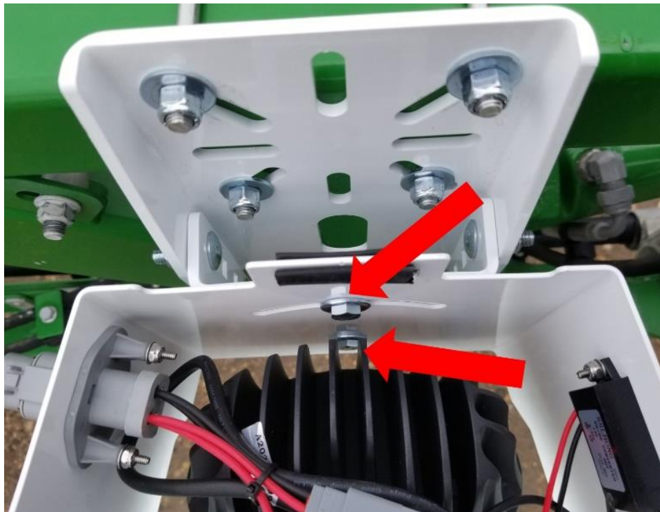
Fig. 17: Fasteners for Pitch Adjustment
