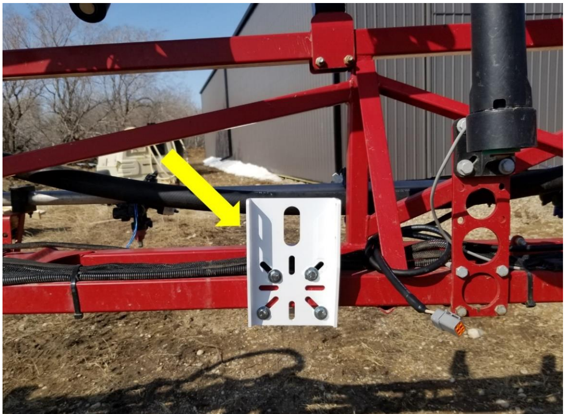
Fig. 4: Mount Location at Bottom of Boom
