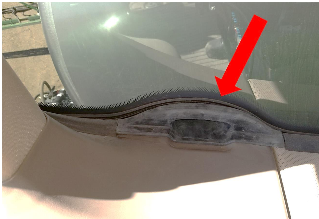
Fig. 11: Entry Grommet at Right Rear Corner of Cab (John Deere)
