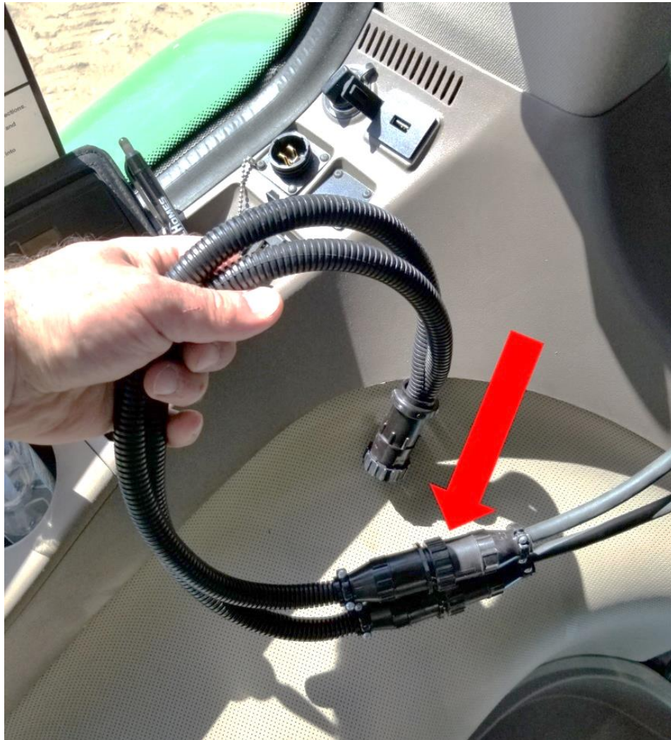
Fig. 14: Power Cable Assemblies Connected to Power Cable Y-Adapter
