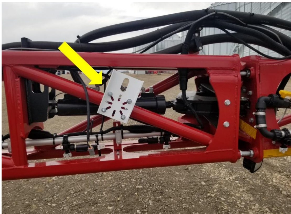
Fig. 5: Mount Location in Center of Boom
