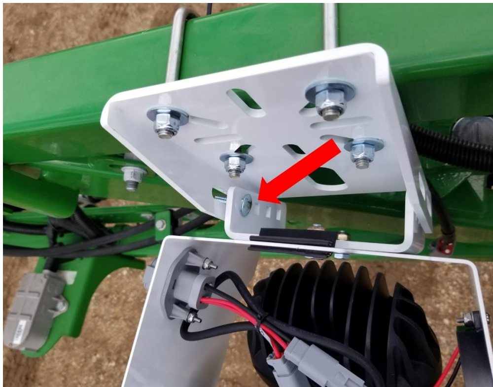
Fig. 6: Initial Upper Carriage Head Bolt Installed
